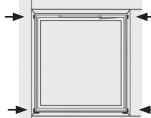
**UK:** Position frame in place according to the predetermined position. Wedge at the bottom of each side (opposing wedges from inside and outside). Side jambs must be plumb and square.
