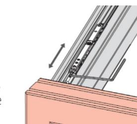
**UK:** When the frame is properly fitted, more adjustments can be done by adjusting fittings in the frame and sash.
