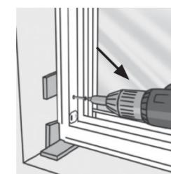
**UK:** Place exactly fitting blocks where the windows fixing holes are positioned, and fix with screws where the predrilled holes are positioned in the frame.
