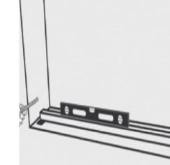
**UK:** Decide and mark the position of the frame in relation to the inner and outer wall.
