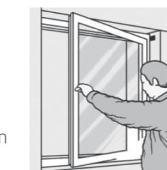
**UK:** Check the gap between frame and sash is even all around. Adjust the frame if necessary. Remove temporary wedges.
