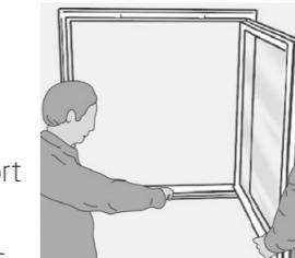
**UK:** Open the sash 90 degrees and support the sash while fixing the frame to the wall. Remove transport blocks.
